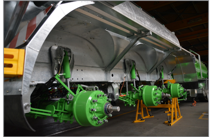
VOLUMETRA 22500 with wheel recessing for large wheels and bolted Hydro-Tandem running gear
